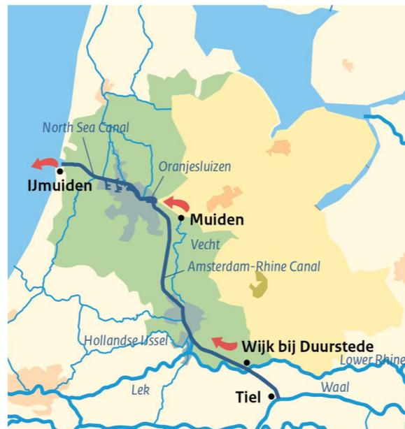
Basin of the Amsterdam-Rhine Canal and the North Sea Canal. The green area shows where the water is directly discharged, the yellow area shows indirect discharge.
