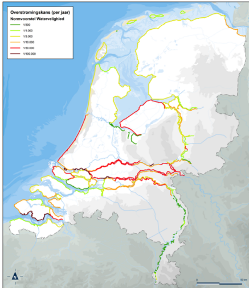
Figure 2.1: Acceptable annual probabilities of failure for future safety assessments in the Netherlands from 2017 (Deltaprogramma, 2014). The warmer colors represent higher target reliabilities.
