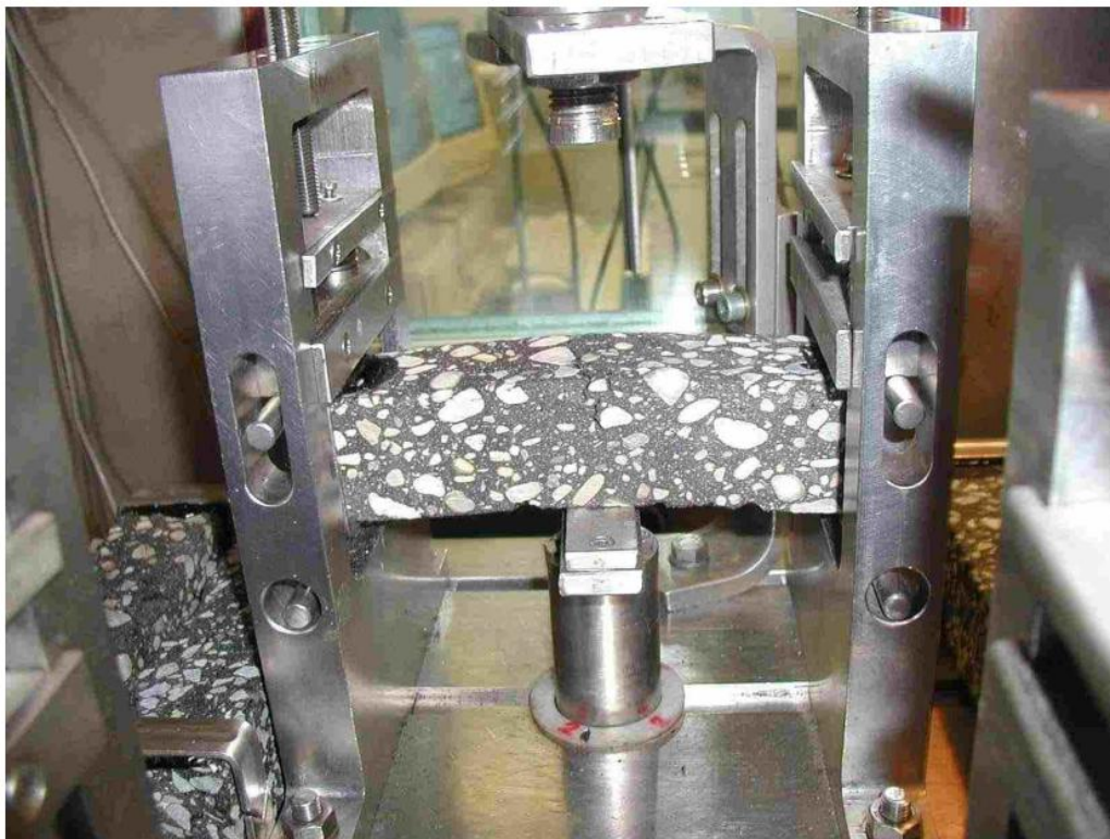
Figure 2.5 Start of yielding of asphaltic concrete in 3 point bending test: a large crack has occurred (see top middle part of asphalt sample)
