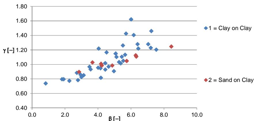
Figure J.6. Influence of the marine or riverine water system on the safety factor  $\gamma_n$  – reliability index relationship.
