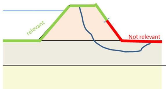
Figure 7.1 Relevant slip circles: slip circles that enter in the green zone are deemed relevant for the flood risk.
