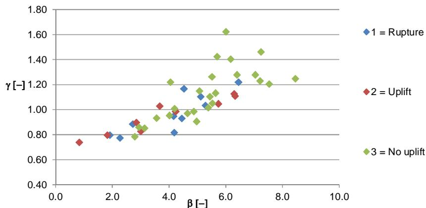
Figure J.7  $\gamma_n$  versus reliability separated in uplift or non-uplift for the WBN.
