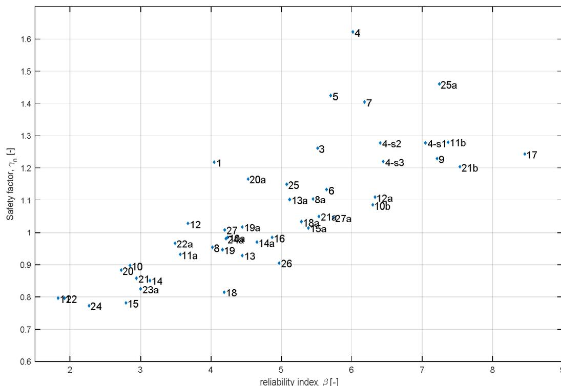
Figure 8.1 Test case results showing the computed  $FoS_{des} / \gamma_d = \gamma_n$  and computed reliability indices for the 2016 test set.
