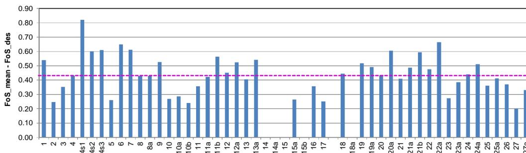
Figure H.1 Difference between Factor of Safety for mean values and Factor of Safety based on design values, and correspondent mean value.
