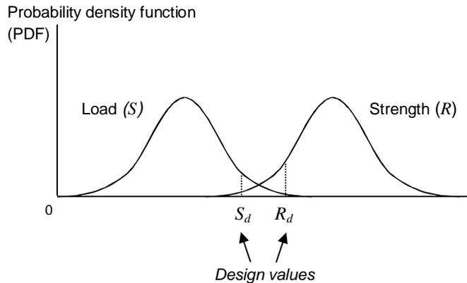
Figure 2.1. Probability density function of load ( $S$ ) and strength ( $R$ ), and the correspondent design values  $S_d$  and  $R_d$ .
