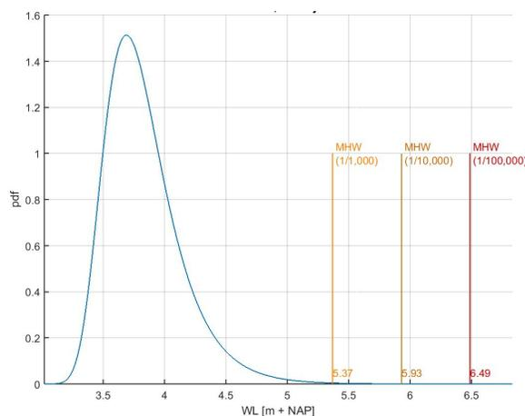
Figure J.1 Example of a water level distribution and the corresponding WBNs for the return periods of 1/1,000, 1/10,000 and 1/100,000.
