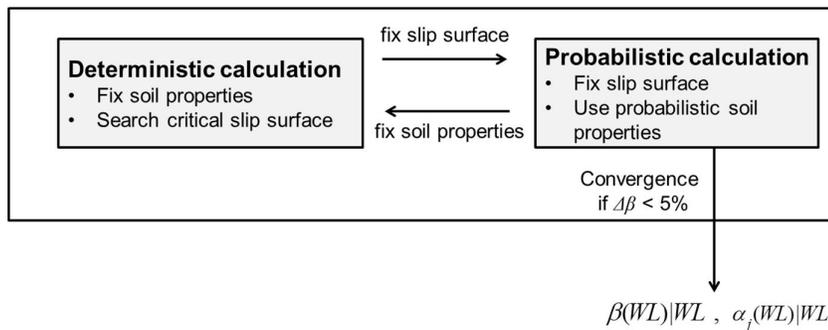
Figure A.1 Calculation scheme of the conditional reliability index  $\beta(WL) | WL$  and of the conditional sensitivity factor  $\alpha(WL)|WL$  for different water levels.
