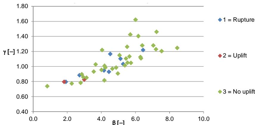
Figure J.8  $\gamma_n$  versus reliability separated in uplift or non-uplift for the water level in the design point.
