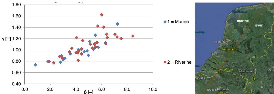
Figure J.4. Influence of the marine or riverine sub-soil on the safety factor  $\gamma_n$  – reliability index relationship (left figure). Separation in marine (west) and river (east) (right figure)
