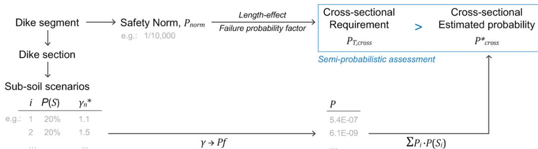
Figure 9.1 Schematised semi-probabilistic assessment for the slope stability mechanism in the WBI 2017 (as in Jongejan & Klerk (2015)).
