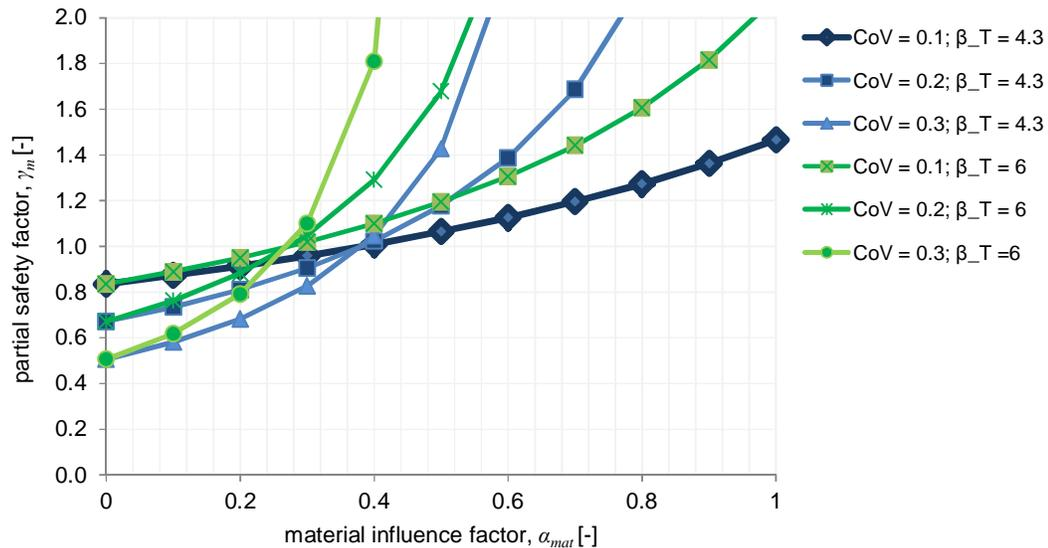
Figure 6.3 Relation material factor ( $\gamma_m$ ) and sensitivity coefficients ( $\alpha_{mat}$ )
