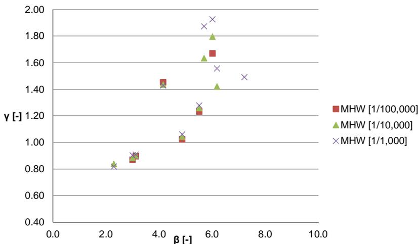
Figure J.2. Influence of the safety level on the safety factor  $\gamma_n$ .
