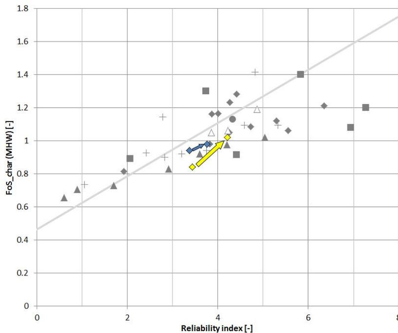
Figure E.1 Calibration fit (grey) with the calibration points of two cross-sections, with and without traffic load based on Kanning et al (2015).
