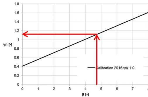
Figure 9.4 Derivation of the required factor of safety, given a target reliability.
