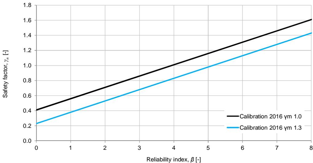
Figure 8.6 Comparison overall safety factor with a material factor of 1.0 and 1.3
