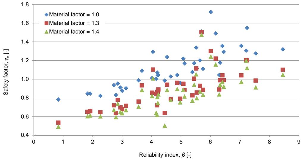
Figure 8.5 Effect of material factors on calculated safety factor
