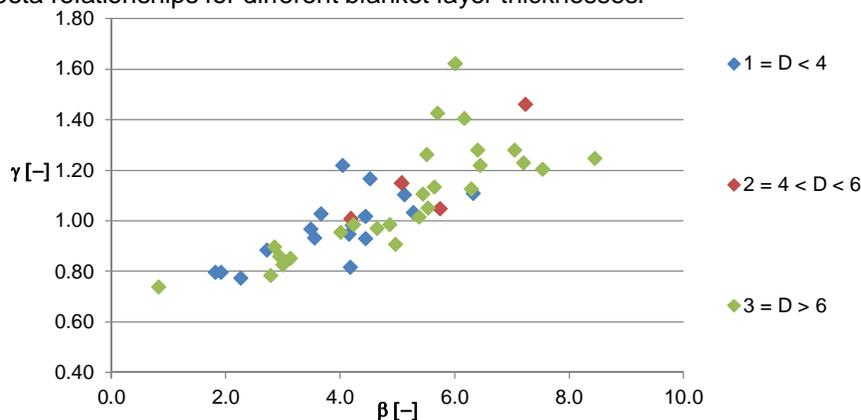
Figure J.9  $\gamma_n$  versus reliability separated for different blanket thicknesses.
