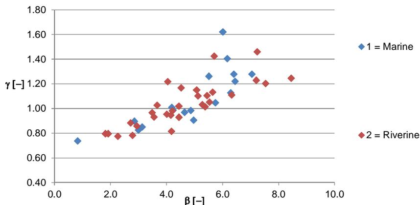
Figure J.5. Influence of the marine or riverine water system on the safety factor  $\gamma_n$  – reliability index relationship.
