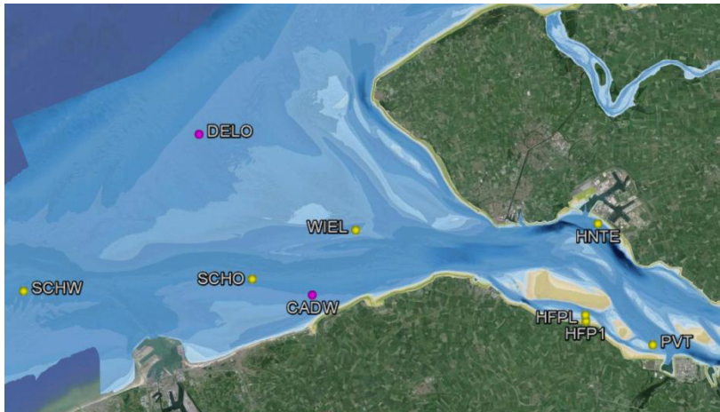
Figure 2.11 Wave measurement locations in the Western Scheldt. The directional wave measurement locations are shown with magenta dots.
