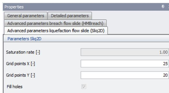
**Figure 3.15:** Advanced parameters liquefaction flow slide (Sliq2D)
