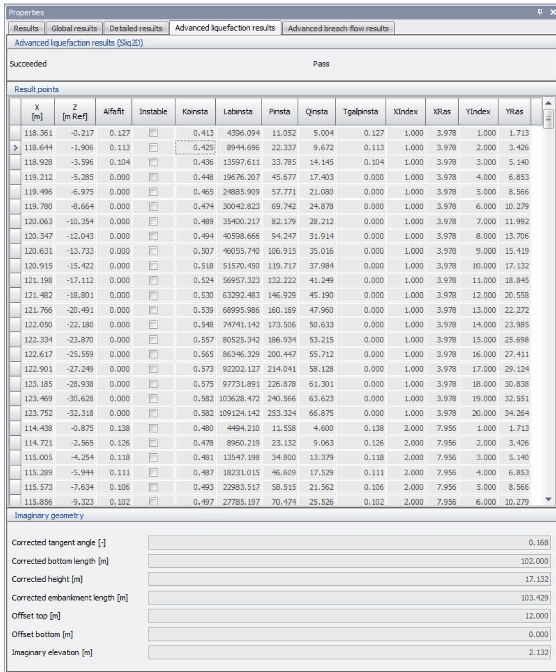
Figure 3.21: Advanced liquefaction results
