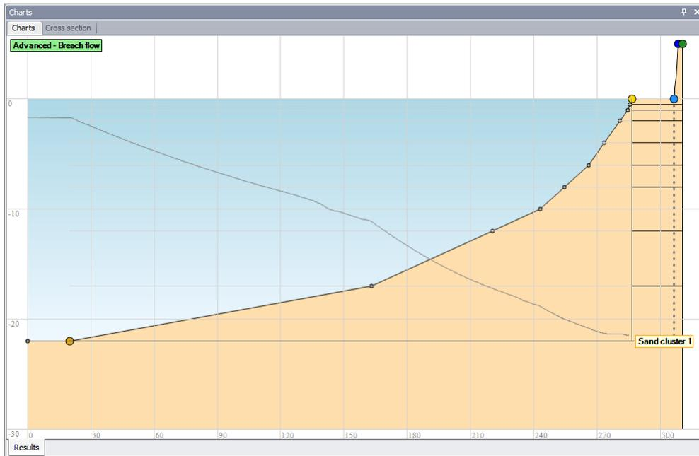
Figure 3.28: Chart after an Advanced Breach flow (HMBreach) check
