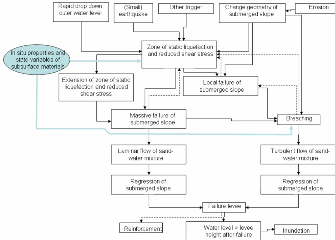
**Figure 1.2:** Processes possibly involved in a flow slide
