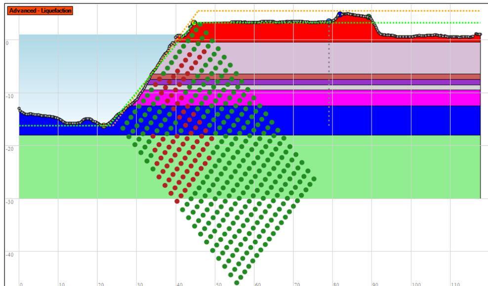
**Figure 3.27:** Chart after an Advanced Liquefaction (Sliq2D) check
