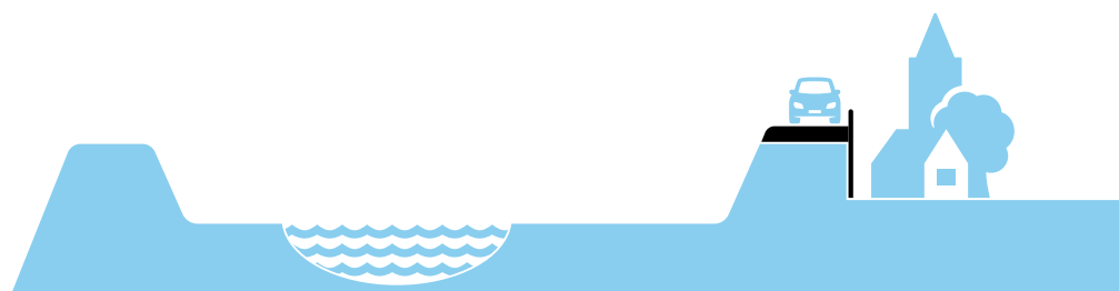
Incorporation - e.g. dyke reinforcement, taking into consideration existing use
