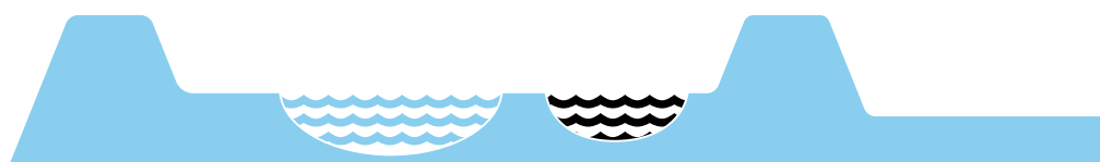
River widening - instead of dyke reinforcement
