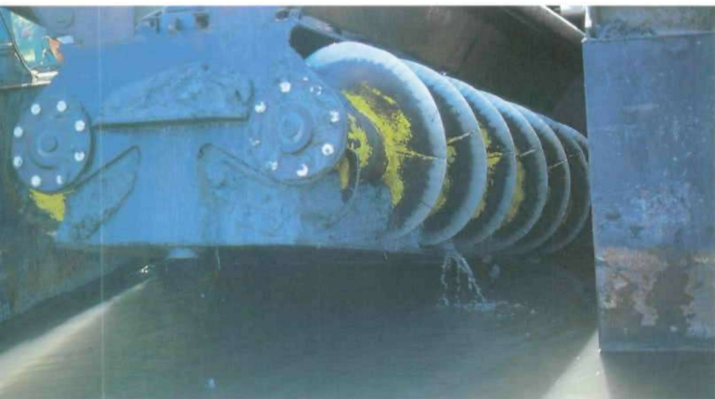
POSW has also conducted dredging tests with a wormwheel suction cutter
